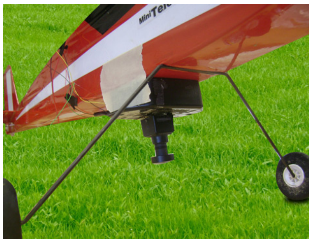
Fig. 3 The IMU and camera setup as mounted on the radio controlled plane.
